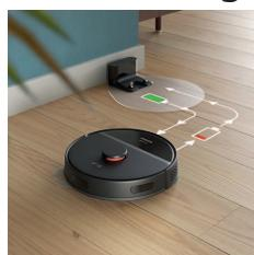
When the battery runs low (<20%) while cleaning, the robot automatically returns to the station to recharge. After the battery has been charged, the robot continues where it has left off.
