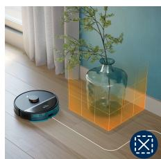
**i** Note: The robot can get stuck on high pile carpets, carpets with fringes or very light rugs like in the bathroom. Also the robot cannot detect cables on the floor.
